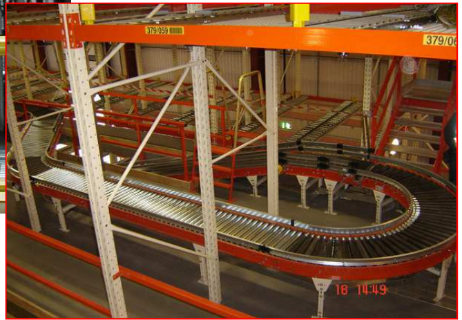
TRAVIROLL® : dynamic storage on TRAVIRACK® pallet racking.
