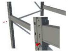
Front: the strongest (highest) beam is installed at the front.
