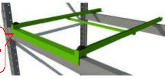
Both the front and back beam have to be bolted to the upright.
