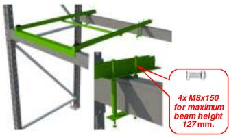
Attach the bottom section to the rear beam by means of the supplied brackets. The width of the bottom part is 800 mm and this part needs to be correctly spaced across the beam length.
