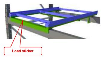
Once the top section has been installed, the flange prevents backward rolling out of the C-profile. Now apply the sticker with the maximum load.
