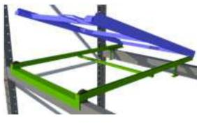
The top part is placed by pulling that part through the C-profiles at the back.
