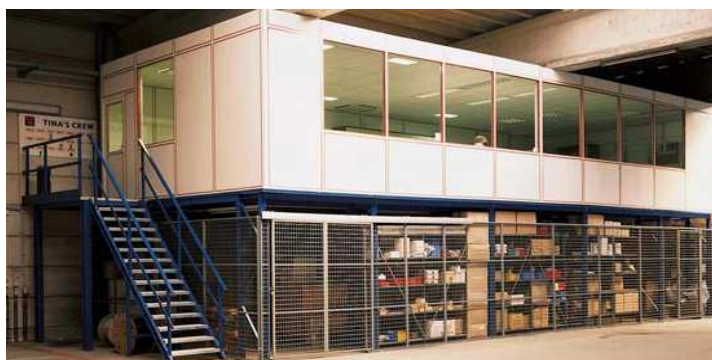
Mezzanine built on TraviRack® columns with Cornix Plus® shelving below secured by CORNIX® mesh partitioning and ALUMEL office partitioning upstairs.
