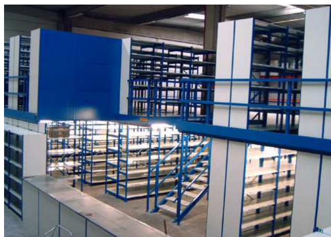
CORMAG® sales counter integrated in a multi tier CORNIX PLUS® shelving installation with display shelving as an extension of the sales counter (installation being built by the CORNIX installation team).
